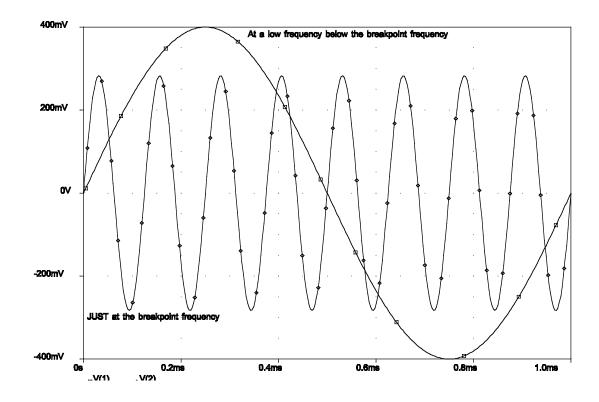
3) At the breakpoint frequency, the amplitude of the output voltage will drop by 3 dB (i.e. it will drop to  $(0.5)^5 = 0.707$  of its value in the passband. Using 4 divisions as the passband value, 4 divisions (0.707) = 2.83 divisions at the breakpoint frequency.
